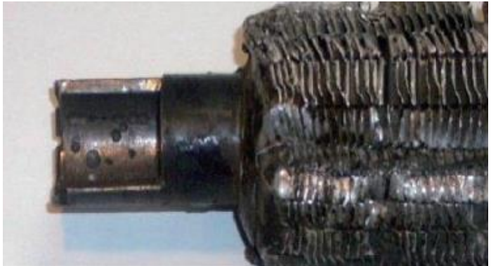
점식 (Pitting Attack)
